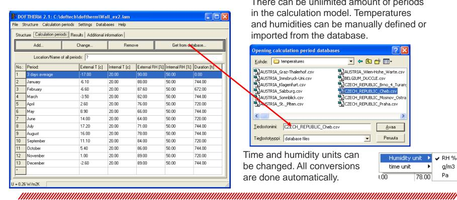
There can be unlimited amount of periods in the calculation model. Temperatures and humidities can be manually defined or imported from the database.
