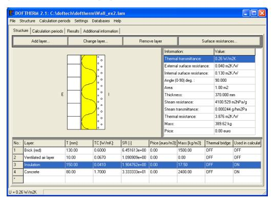
DOF-THERM provides an easy and fast way to calculate the thermal transmittance (U-value) together with temperature and humidity curves.
