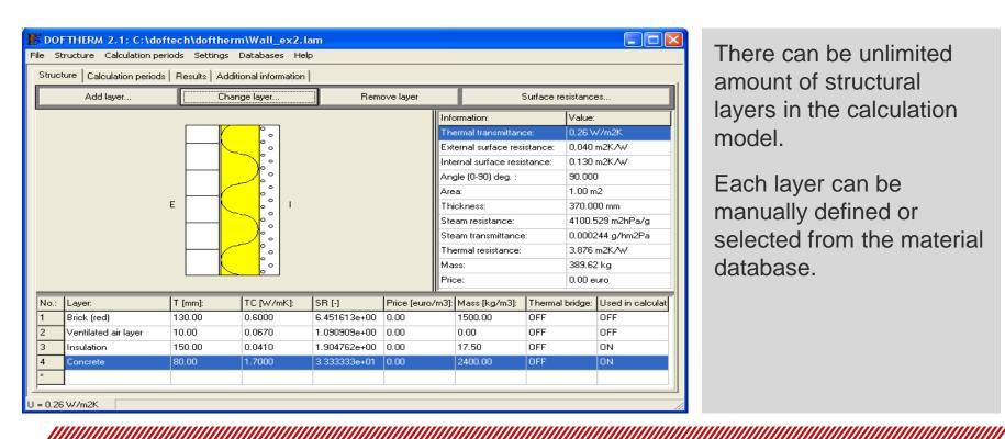
There can be unlimited amount of structural layers in the calculation model.
